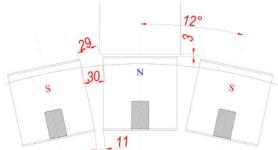
The drawing on the left shows a diagram of the interaction of magnets taking into account their overall dimensions and the minimum distances required to ensure the strength and rigidity of the flywheel system with magnets. Based on this arrangement, we will construct a flywheel drawing for further calculations.
