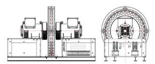
The drawing shows an electric generator that uses magnetic force to rotate alternator rotors. The drawing shows one disk, but multiple disks can be used to increase power.
